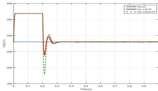
Fig. 7. Dc link voltage when connected to the network
