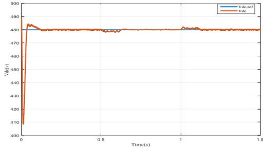
Fig. 6. Dc link voltage using feed compensator
