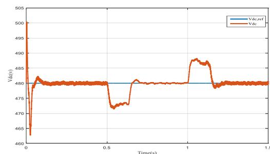
Fig. 5. Dc link voltage without the use of a feed compensator
