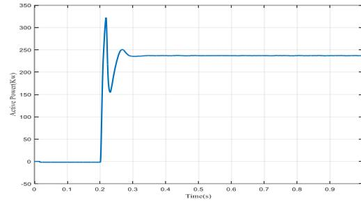
Fig. 9. Active output power of the photovoltaic system when connected to the grid
