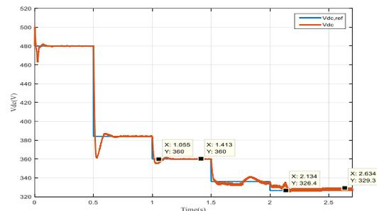
Fig. 18. Reference voltage of dc link
