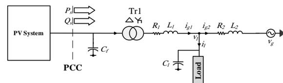
Fig. 2. Single-line diagram of PV system in connection to distribution network
