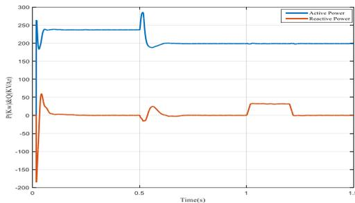
Fig. 16. Active and reactive power System output in independent control of active and reactive power
