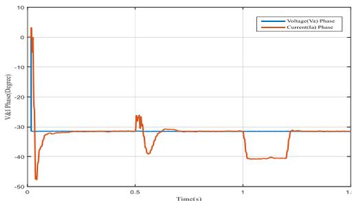
Fig. 17. PCC line current and voltage phase in independent control of active and reactive capacities
