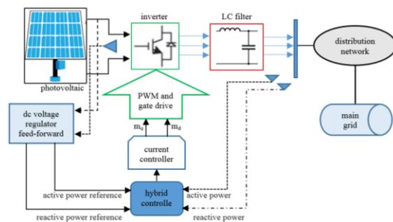
Fig. 3. The PV system studied in the network connection mode
