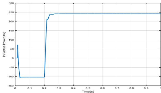
Fig. 8. Active output power of a photovoltaic panel array when connected to the grid
