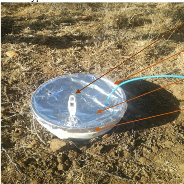
**Fig. 2.** Static GHG chamber
