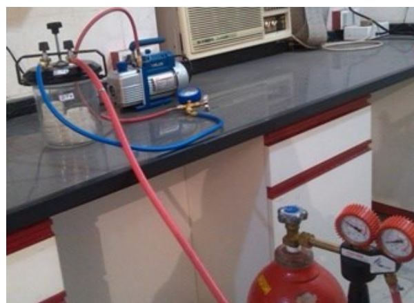
Fig 1. The apparatus that was used for obtaining 50% methane and 50% air for bacterial growth (9, 15).
