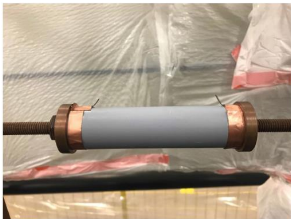
Fig. 13. SIR Sample with Pre-stressing setup.
