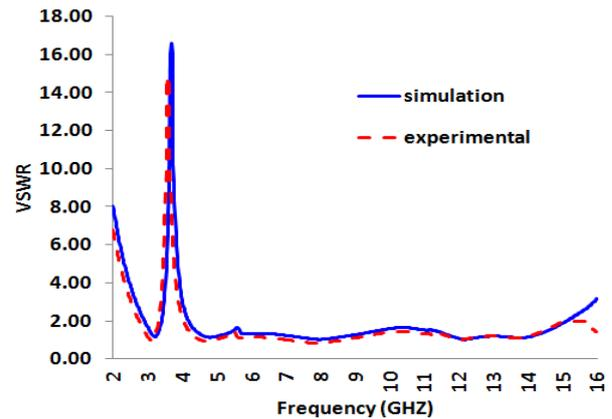
**Fig.2. Simulation and experimental results of the VSWR.**
