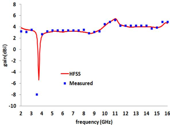
Fig. 4. The simulated and measured antenna gain.
