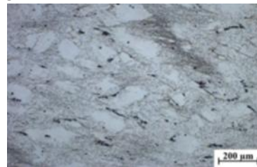
Figure 9- Micro-structure after forging [10]
