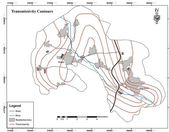
Fig. 5. Groundwater transmissivity of the study area
