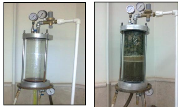
Fig. 3. Schematic view of the built filter device
