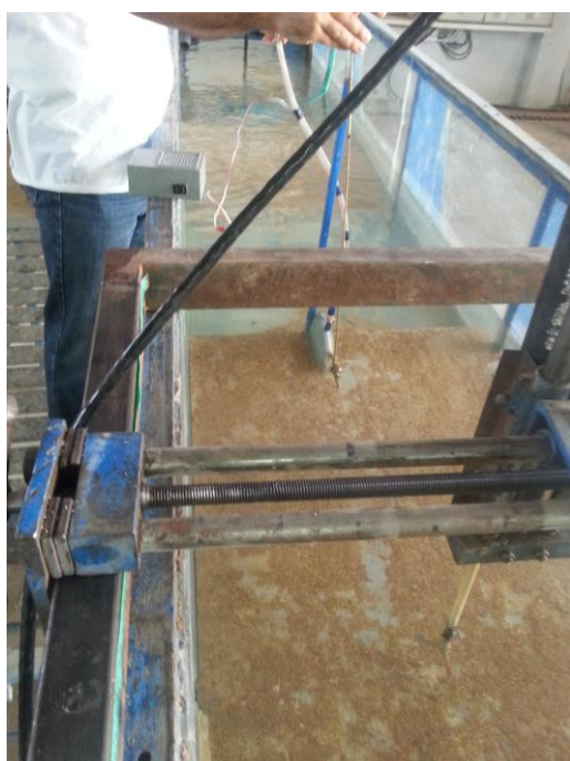
Fig. 4. Calibration setup for VCM device in the flume
