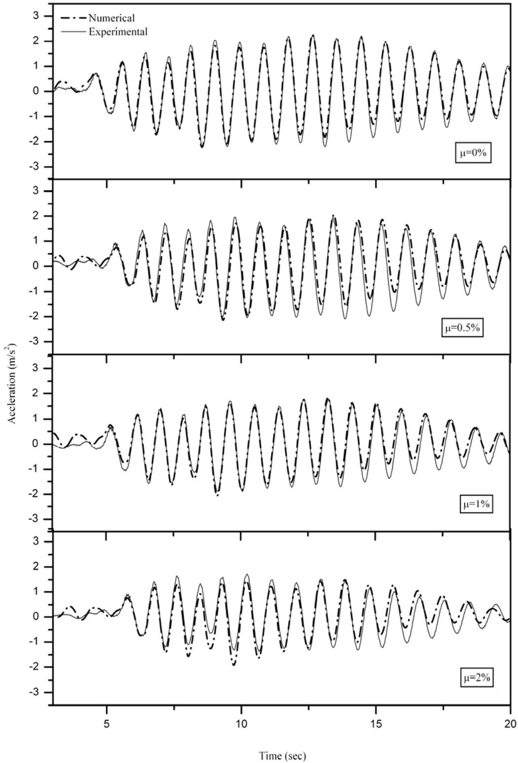
Figure 9. Comparison between numerical and experimental structural acceleration time histories for a structure (Case 1:  $T_s=0.9s$ ) with TLD ( $\Delta=0.077$ ) subjected to a typical artificial ground time history
