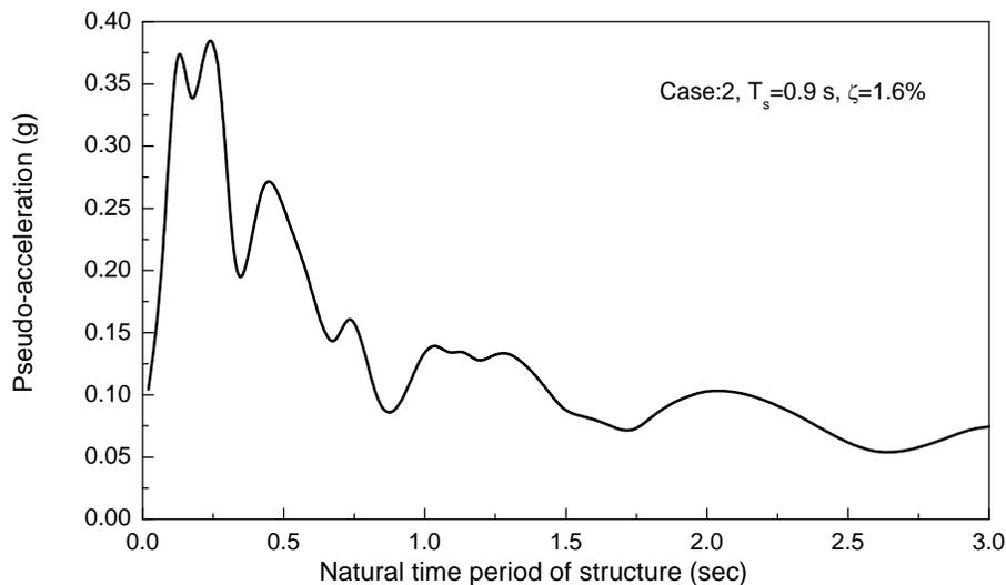
Figure 3. Typical plot of individual response spectra of artificially generated ground time-histories used for shaking table experiments (Case2)
