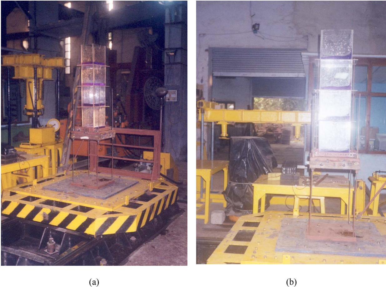
Figure 2. a) test setup, specimen and shaking table; and b) behavior of liquid inside TLD during the test
