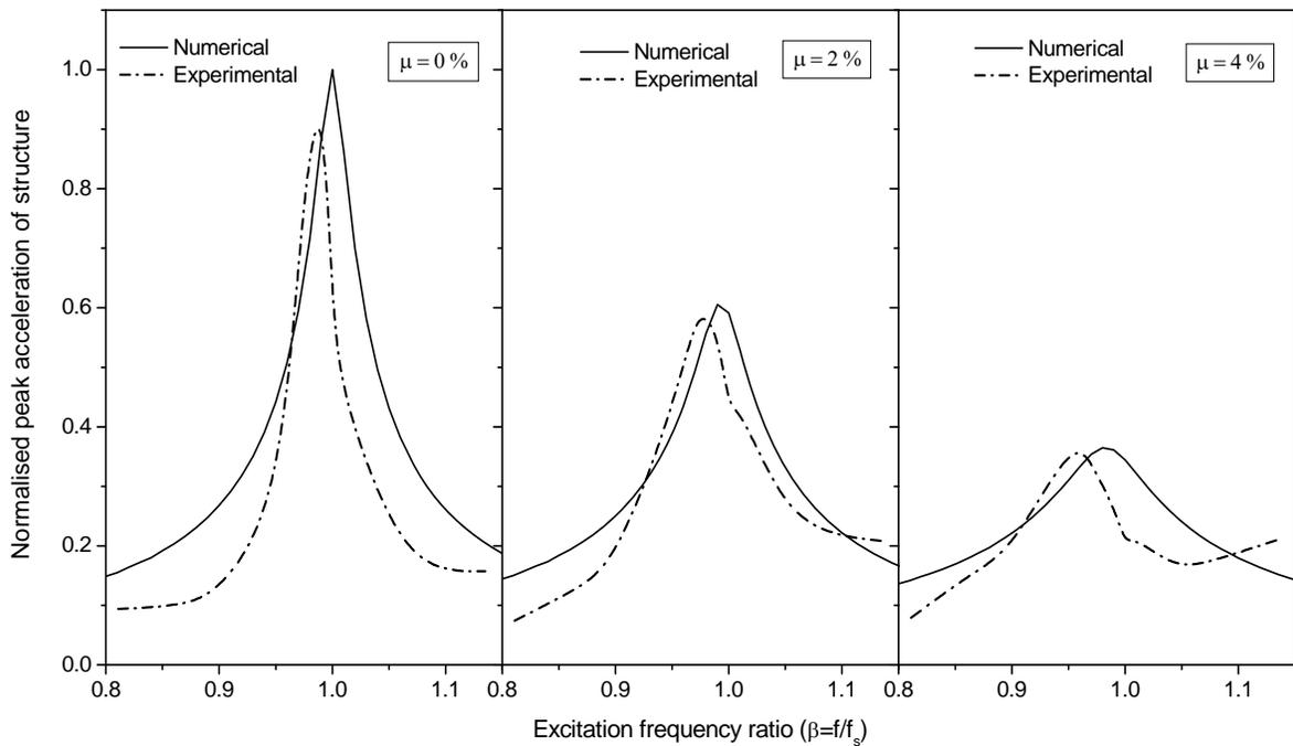
Figure 8. Normalized peak acceleration for different mass ratio and varied  $\beta$  ratio (Structural type: Case 4,  $T_s=0.9s$ ,  $\Delta=0.151$ ,  $A_0=0.0963 \text{ m/sec}^2$ )
