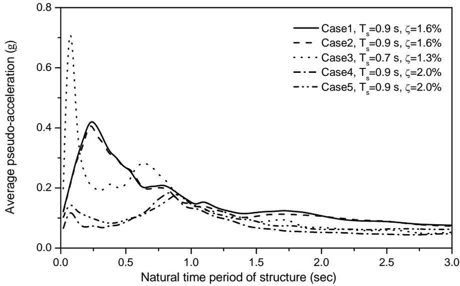
Figure 4. Average response spectra of artificially generated ground time-histories used for shaking table experiments for all five cases
