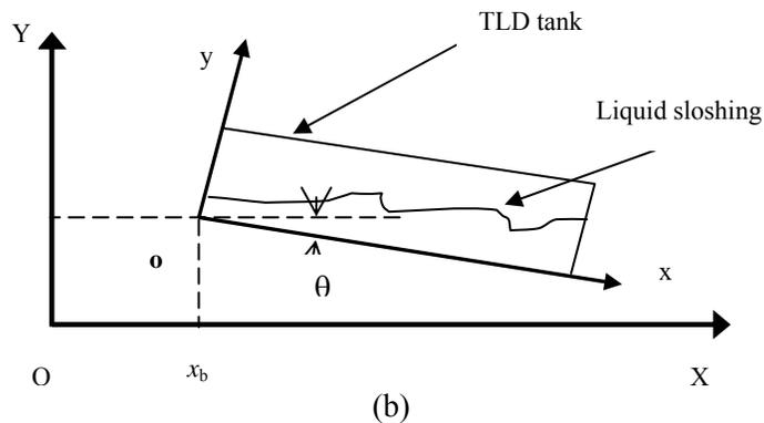
Figure 5. Schematic diagrams of TLD tank and liquid sloshing inside it under coupled horizontal and rotational motion
