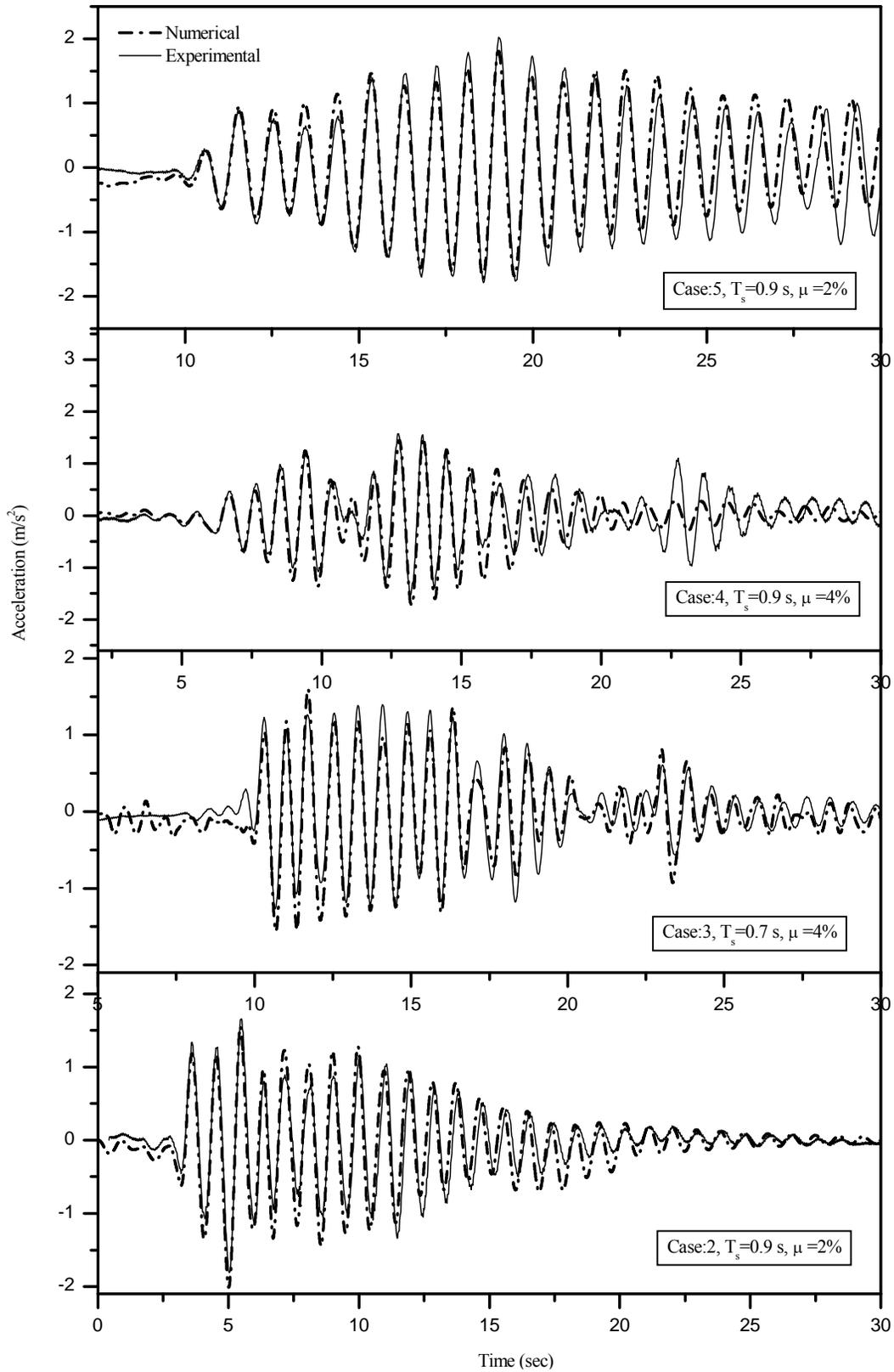
Figure 10. Comparison between numerical and experimental structural acceleration time histories of different structures attached with TLD subjected to typical base excitation
