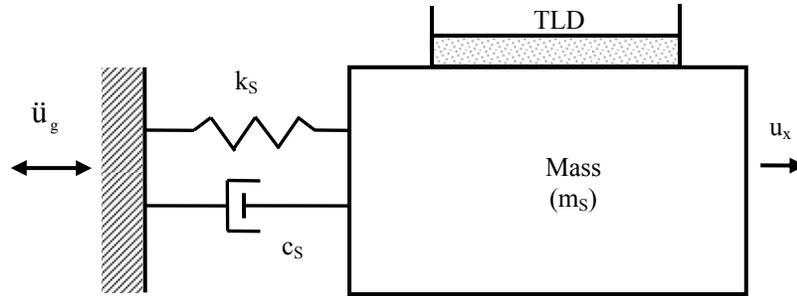
Figure 6. Schematic diagram of a single-degree-of-freedom shear beam structure with a rectangular tuned liquid damper
