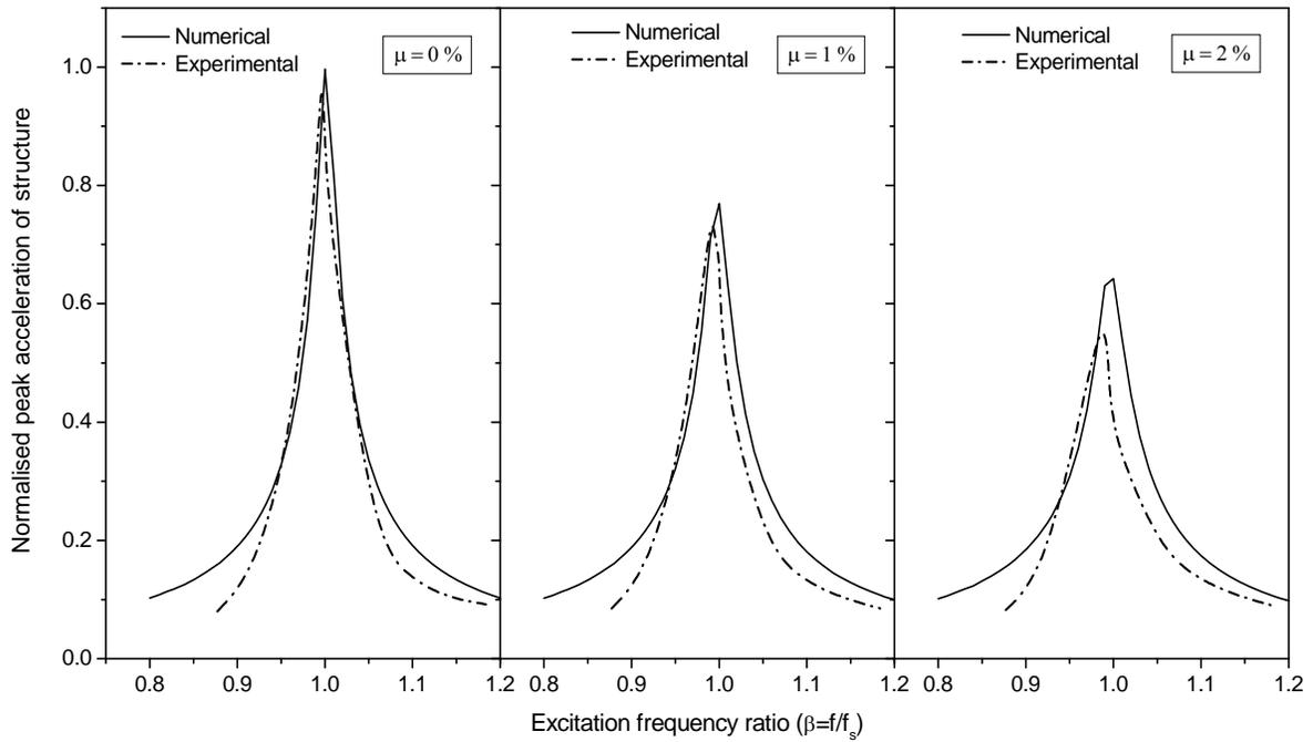
Figure 7. Normalized peak acceleration for different mass ratio and varied  $\beta$  ratio (Structural type: Case 1,  $T_s=0.9s$ ,  $\Delta=0.077$ ,  $A_0=0.053 \text{ m/sec}^2$ )
