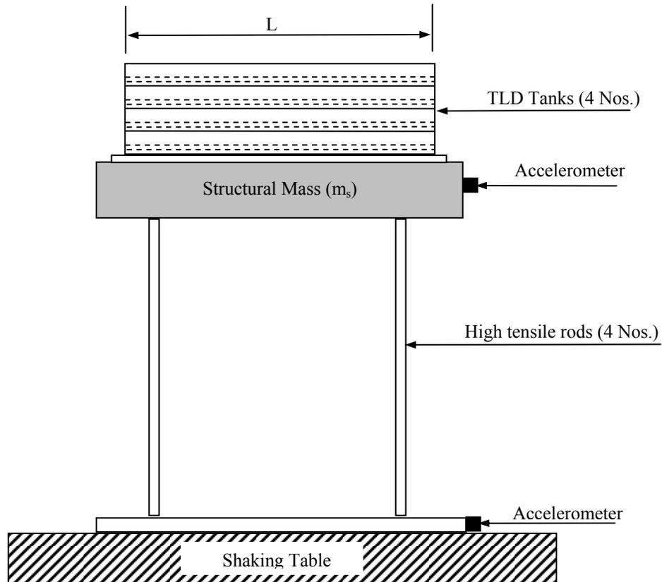
Figure 1. Schematic diagram of TLD-structure model
