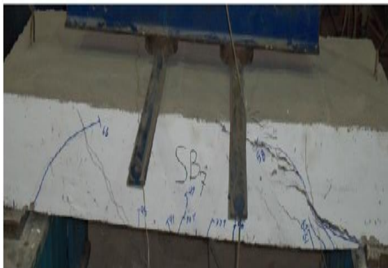
Fig. 6. Sample crack pattern SB7 [22].
