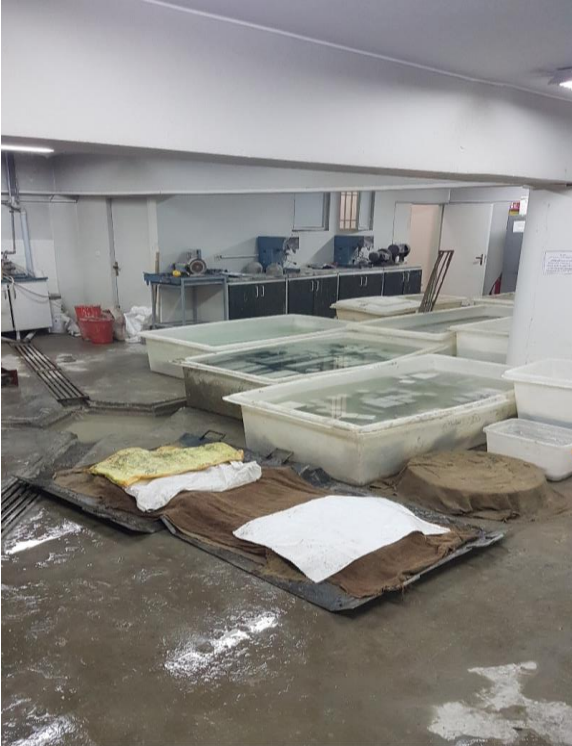
Figure 4: Preparing and curing of fiber concrete samples
