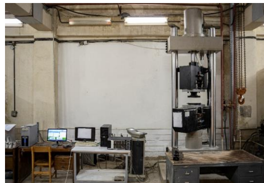
Figure 7: A view of Dartec9600 self-control loading device
