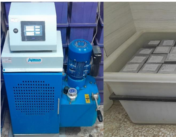
Fig. 6. Compressive strength test machine and concrete curing tank
