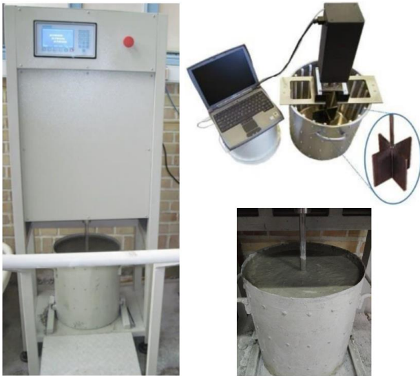
Fig. 5. Rheometer device and tested sample
