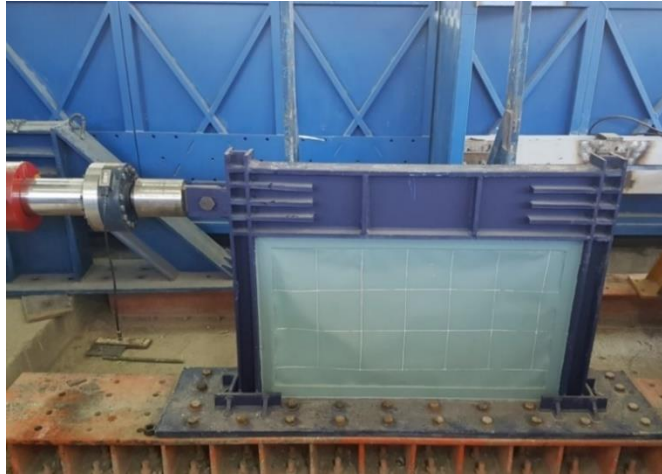
Fig. 4. Initial connection of sample to the bottom chassis and jack.
