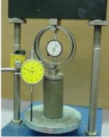
**Figure 2.** Shattering sample in uniaxial device with the addition of 0.8% nanosilica
