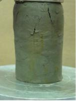
Figure 3. Broken sample in uniaxial device with the addition of 2% Nano-silica
