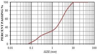
Figure 1. Report of sand grading experiment
