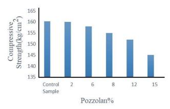
Figure 3. Concrete strength with different percentages of pozzolan with 400 grade cement at 7 days old concrete
