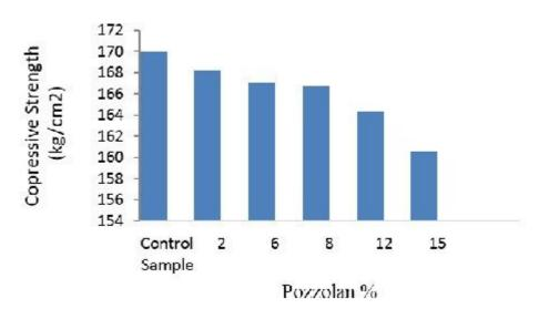
Figure 6. Concrete strength with different percentages of pozzolan with 380 grade cement at 28 days old concrete
