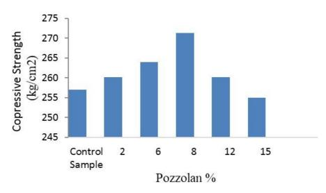
Figure 9. Concrete strength with different percentages of pozzolan with 340 grade cement at 7 days old concrete
