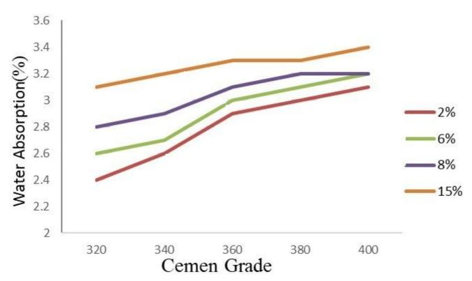
Figure 13. Diagram of water absorption percentage of concrete containing abiotic pozzolan to cement grade
