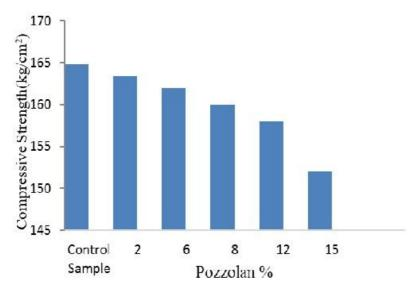
Figure 5. Concrete strength with different percentages of pozzolan with 380 grade cement at 7 days old concrete
