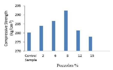
Figure 12. Concrete strength with different percentages of pozzolan with 320 grade cement at 28 days of concrete
