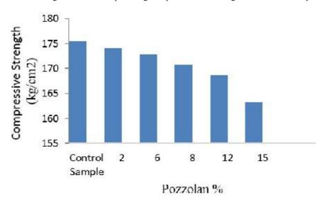
Figure 11. Concrete strength with different percentages of pozzolan with 320 grade cement at the age of 7 days of concrete
