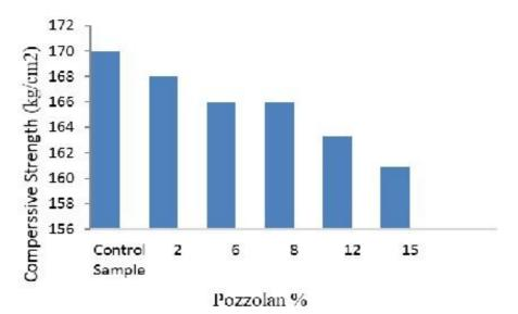
Figure 8. Concrete strength with different percentages of pozzolan with 360 grade cement at 28 days of age
