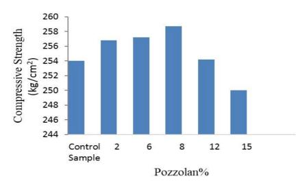
Figure 4. Concrete strength with different percentages of pozzolan with 400 grade cement at 28 days old concrete
