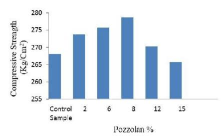
Figure 10. Concrete strength with different percentages of pozzolan with 340 grade cement at 28 days old concrete
