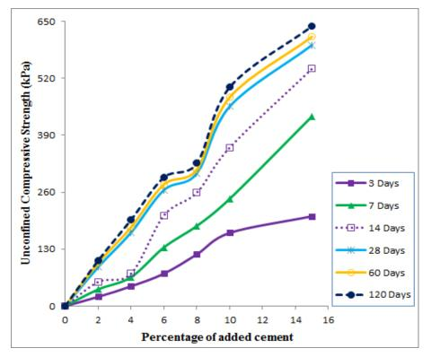
Fig. 7 Changes of compressive strength of the soil sample in different times to the cement ratio
