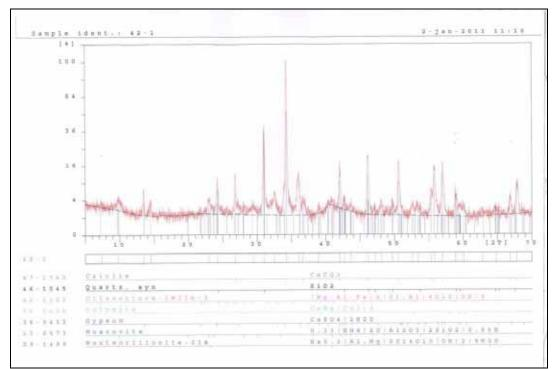
Fig. 4 Characteristic XRD graph of clayey soil (depth of 2.5 m from the trench B)
