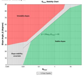
Figure 1. The stability chart for Q-slope (Bar and Barton, 2017)
