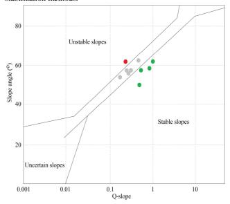
Figure 4. The results of the stability analysis by Q-slope
