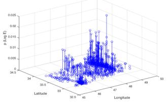
Figure 5. The three-dimensional display of energy probability distribution function for Zagros fault
