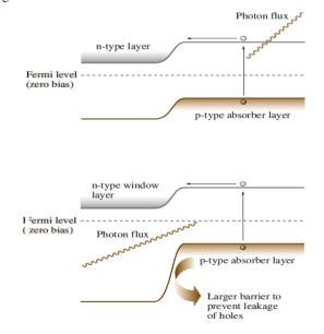
Figure 2. Schematic of an energy-band diagram for a standard solar cell (Kasap and Capper, 2017)
