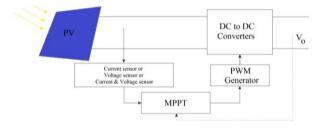
Figure 6. PV mechanism of work
