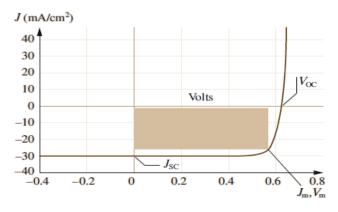
Figure 3. Ideal J–V characteristic for a PV cell
