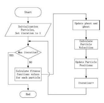
Figure 5. PSO and P&O application flowchart (Qin and Kimball, 2011)
