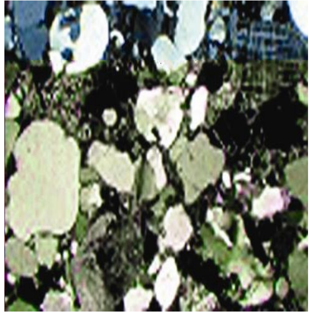
Figure 9. Arkosic wacke with clay cement (X 33)
