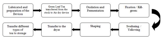
Figure 1. The production process in Soofi Tea Factory.
