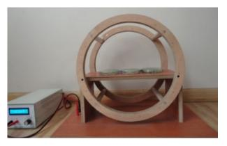
Fig. I. Electromagnetic field exposure arrangement
