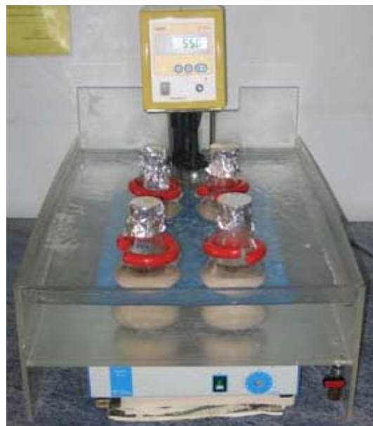
Fig. 1. Experimental set-up used for the extraction of \beta -glucans from barley
