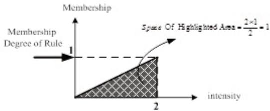
Fig. 9-a. an example of defuzzification
