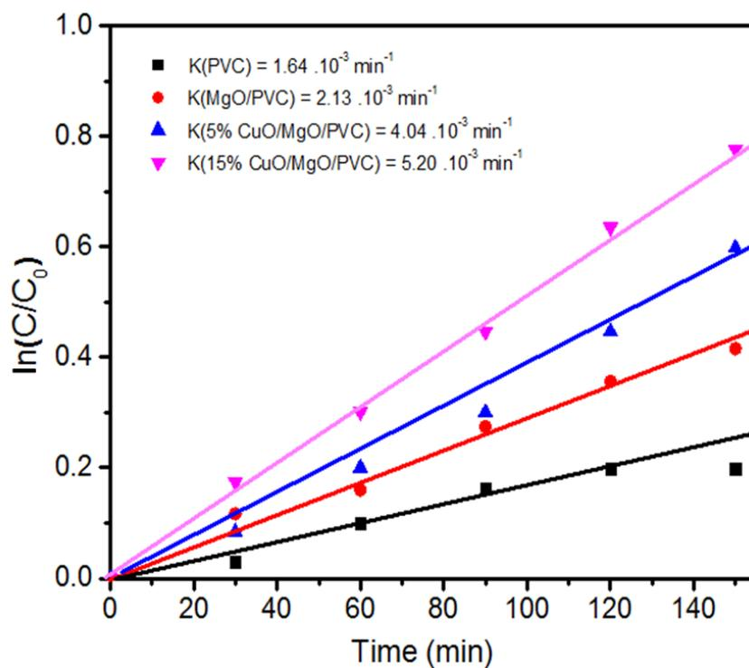
**Fig. 9.** Rate of dye disintegration under,  $[\ln C/C_0]$  vs. time.
