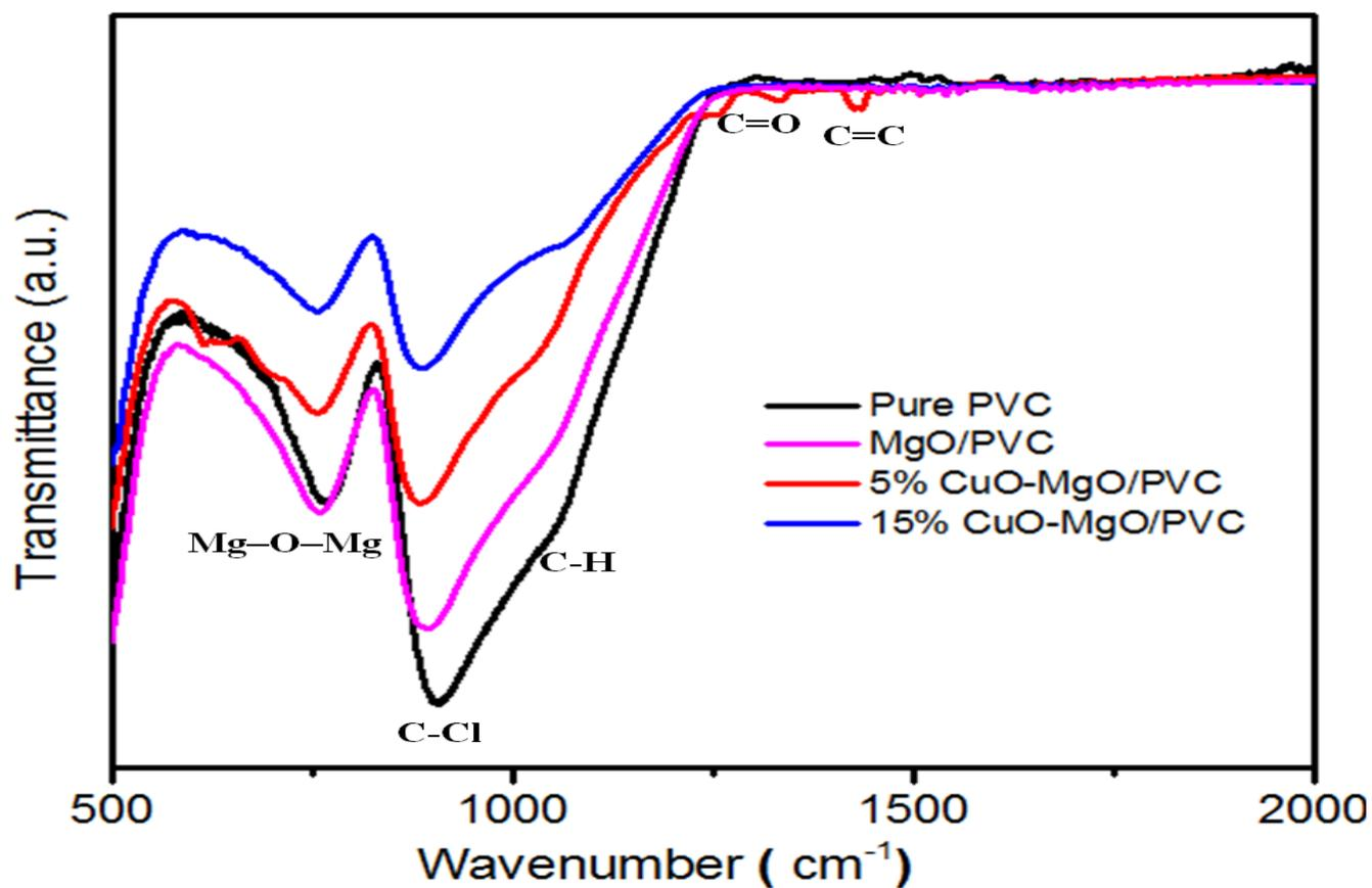
Fig 2. FTIR spectrum of PVC, PVC/MgO, and Cu-MgO/PVC nanocomposites.
