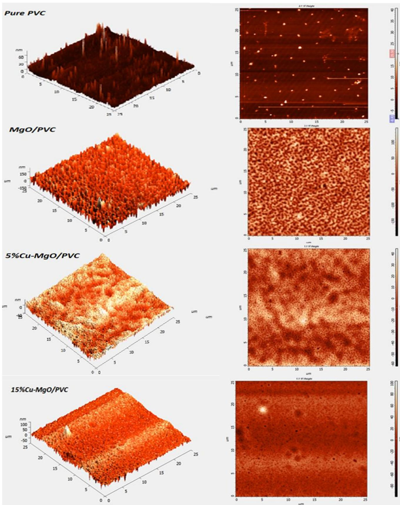
**Fig.7:** AFM for pure PVC, PVC/MgO, and Cu-MgO/PVC nanocomposites.
