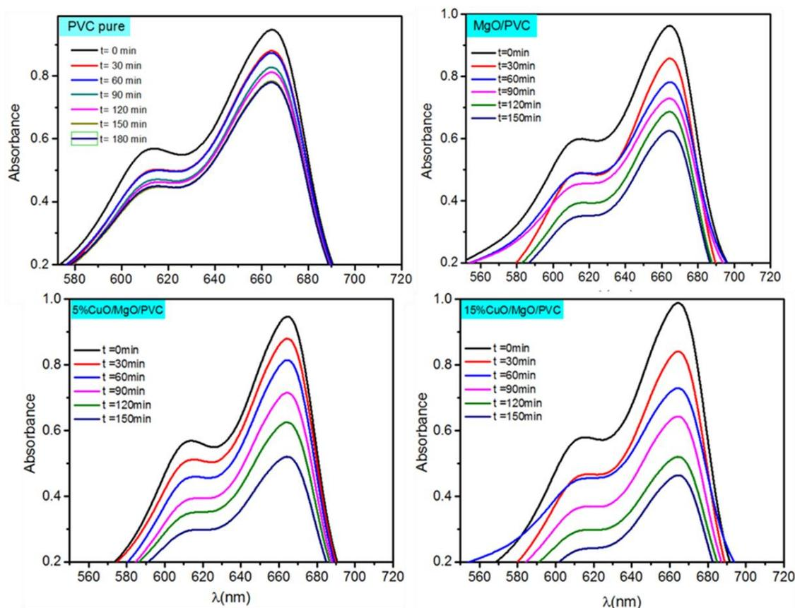
**Fig. 8.** Photocatalytic degradation of MB on exposing to UV light irradiation employing PVC; MgO/PVC and CuO-MgO/PVC heterostructure as catalysts.
