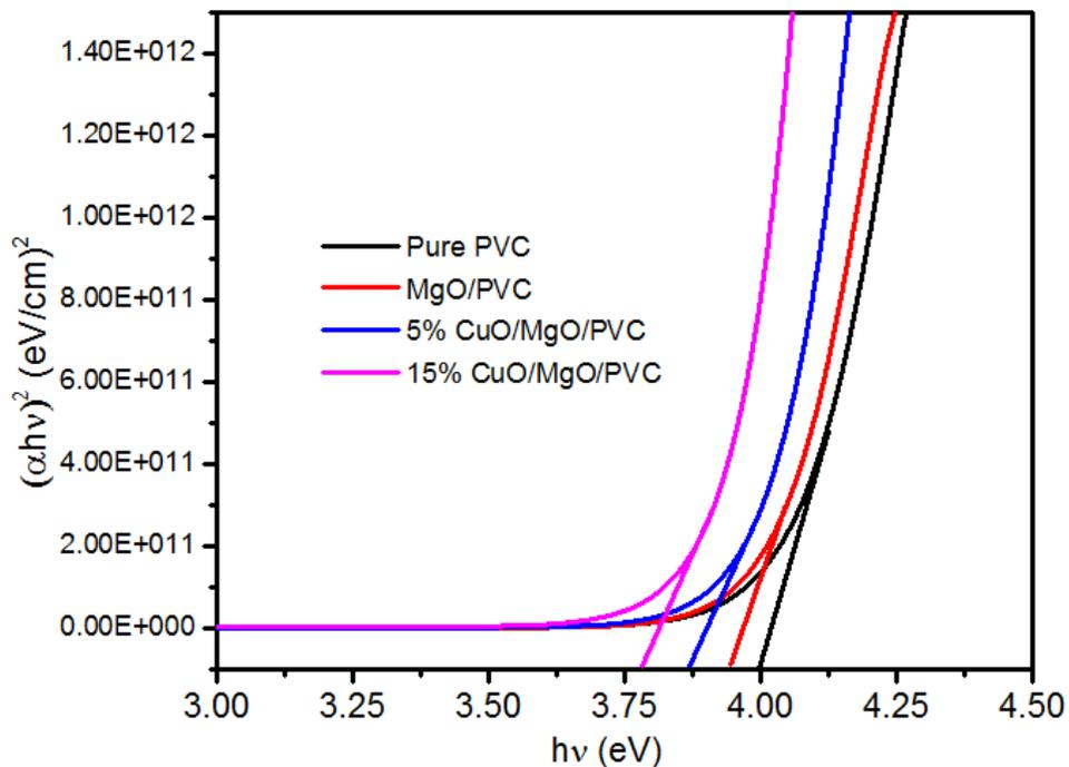
**Fig. 6.** The bandgap of various synthesized nanostructures.
