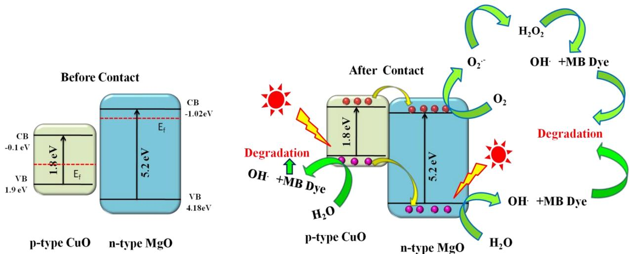
**Scheme 1.** Energy diagram representing p-n heterojunction of CuO/MgO nanocomposites, illustrating separation of electron-hole pairs and bandgap and their involvement in MB dye degradation
