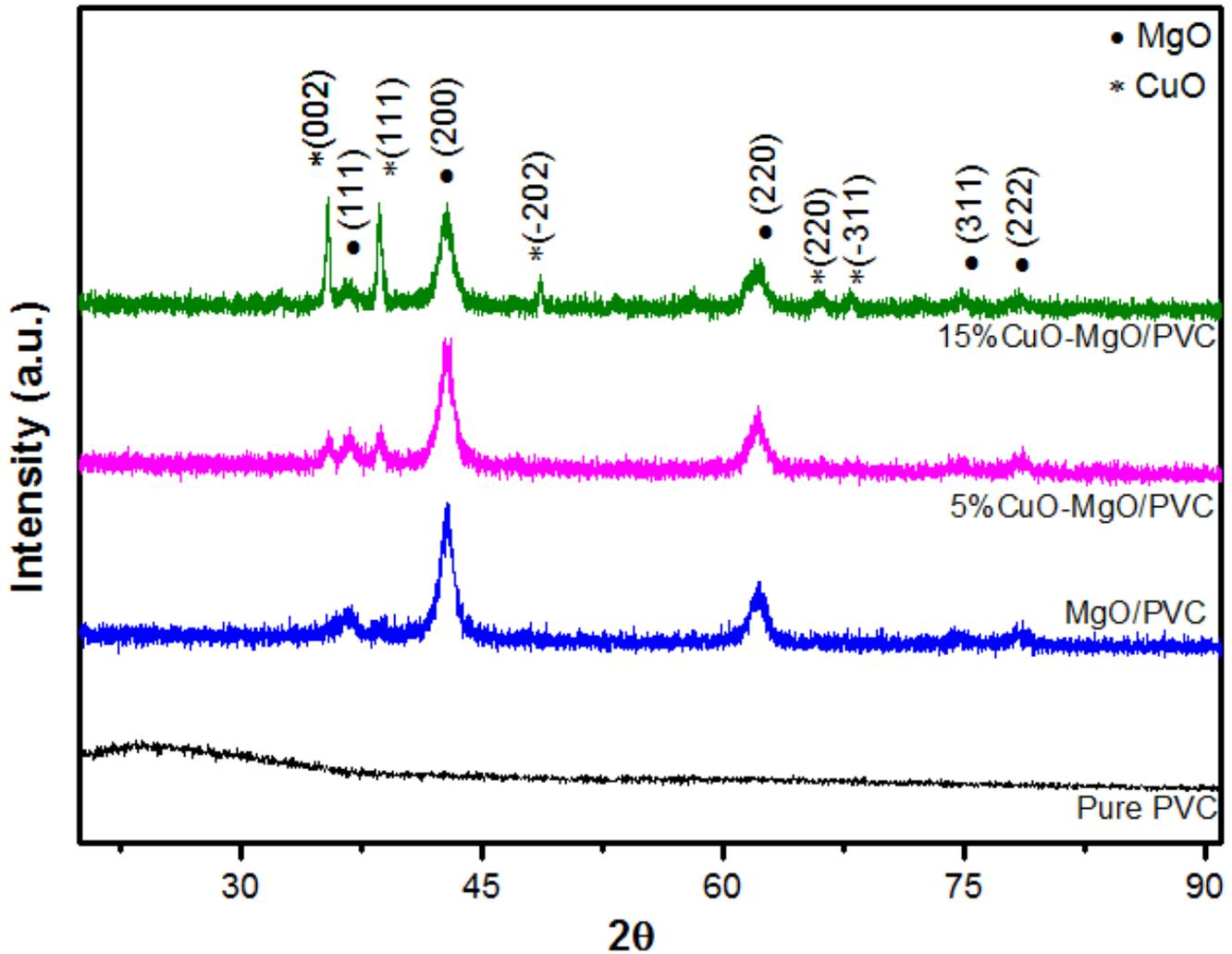
Fig 1. The XRD patterns of Pure PVC, MgO/PVC, and CuO-MgO/PVC nanostructures.
