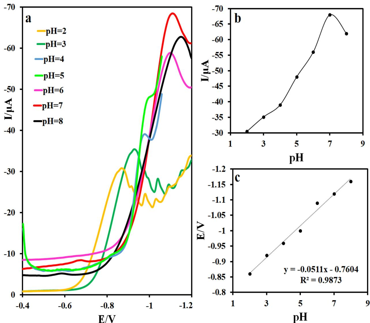
**Fig. 5.** (a) LSV of oxazepam (15  $\mu\text{M}$ ) on the B-RGO/Poly(ASP)|GCE in Britton-Robinson buffer with different pHs at a scan rate of 50 mV/s, (b) I-pH diagram and (c) E-pH diagram
