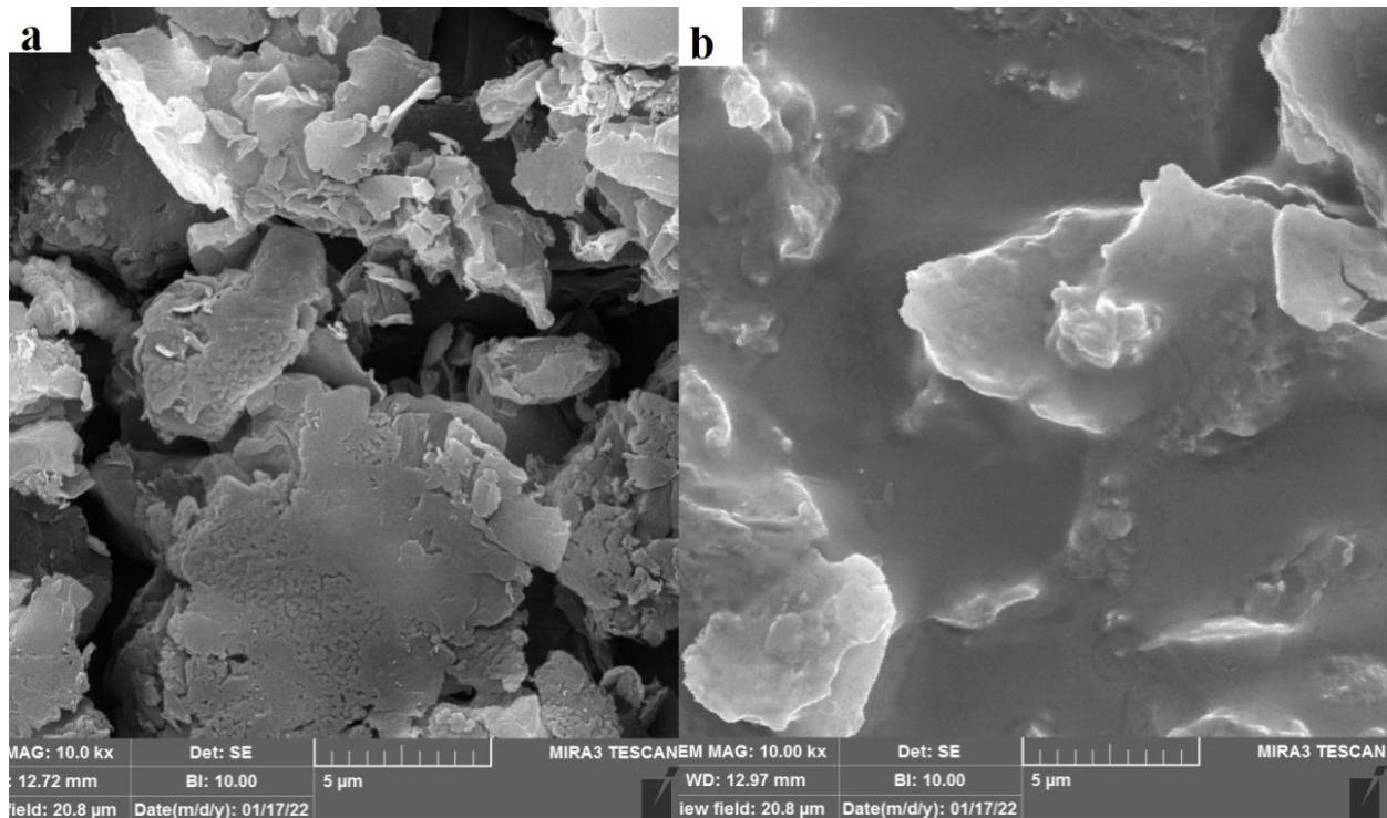
**Fig. 3.** SEM images of (a) B-RGO and (b) B-RGO/Poly(ASP)
