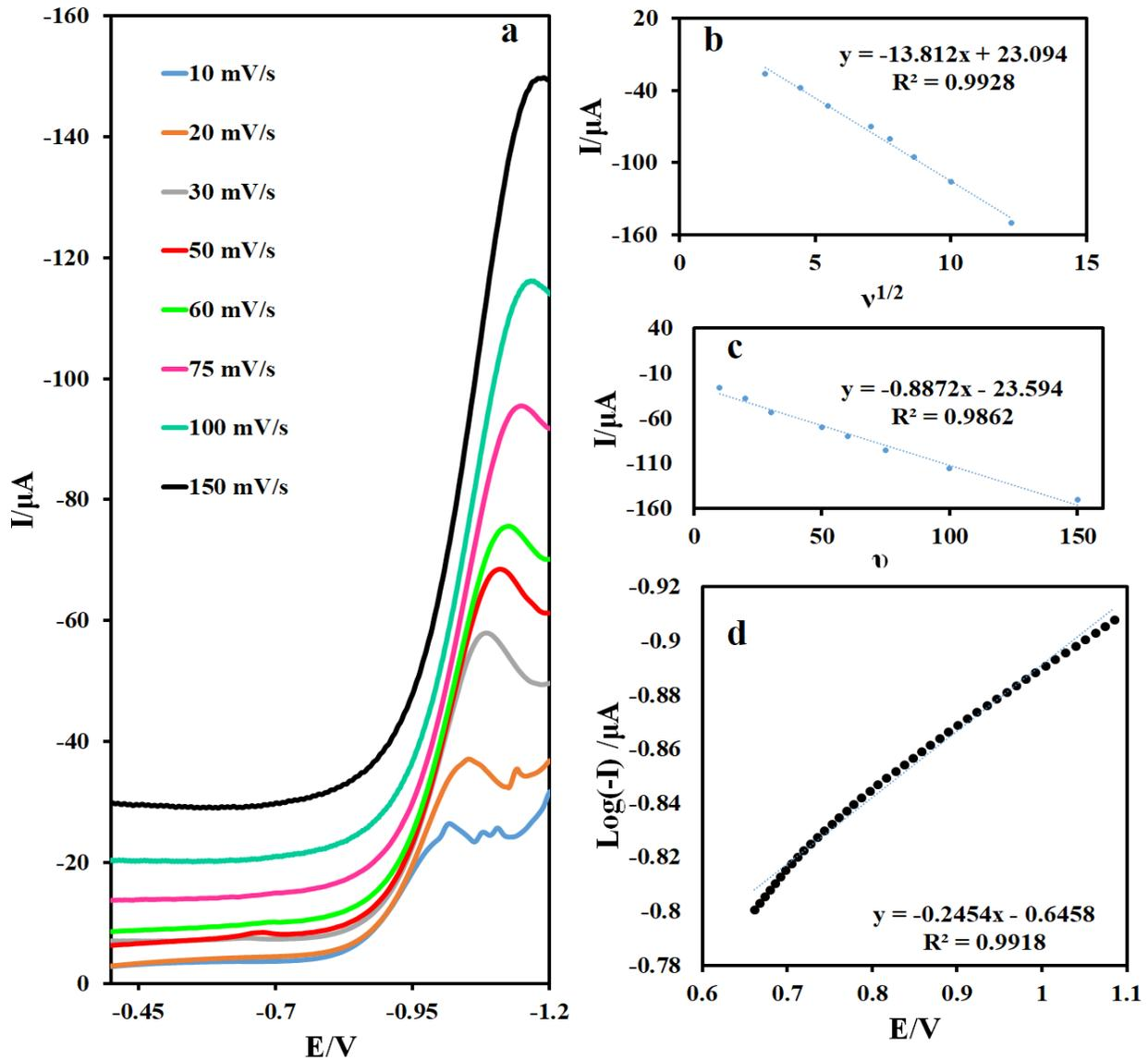
**Fig. 7.** (a) LSV of oxazepam (15  $\mu\text{M}$ ) in Briton-Robinson buffer with pH= 7 at B-RGO/Poly (ASP)|GCE surface at diverse scan rate, (b)  $I$  vs.  $v^{1/2}$ , (c)  $I$  vs.  $v$  and (d)  $\text{Log } I$  vs.  $E$
