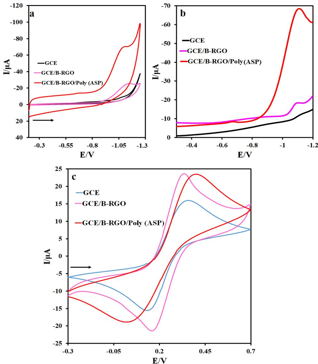
**Fig. 4.** (a) CV and (b) LSV of oxazepam (15 μM) solution on the surface of the different electrodes in Britton-Robinson buffer with pH= 7 at a scan rate of 50 mV/s and (c) CV of hexacyanoferrate probe redox with a concentration of 1 mM in 1 M KNO<sub>3</sub>
