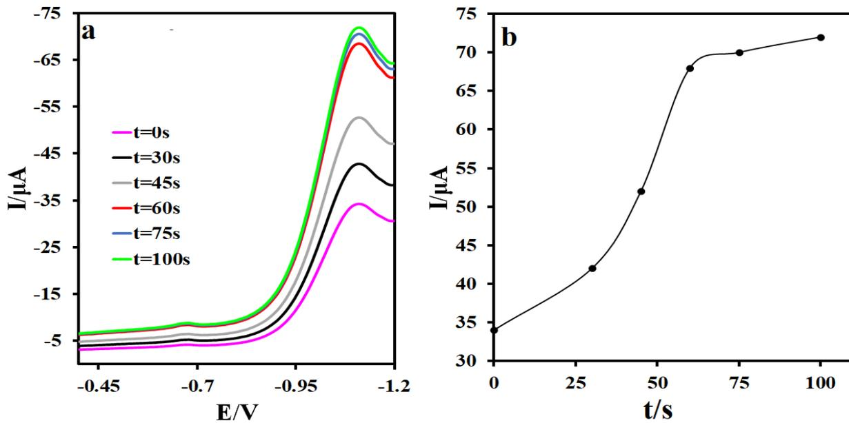
**Fig. 8.** (a) LSV of oxazepam (15 μM) on the B-RGO/Poly(ASP)|GCE surface in the presence of Britton-Robinson buffer electrolyte solution at different times and (b) peak current vs. pre-concentration time
