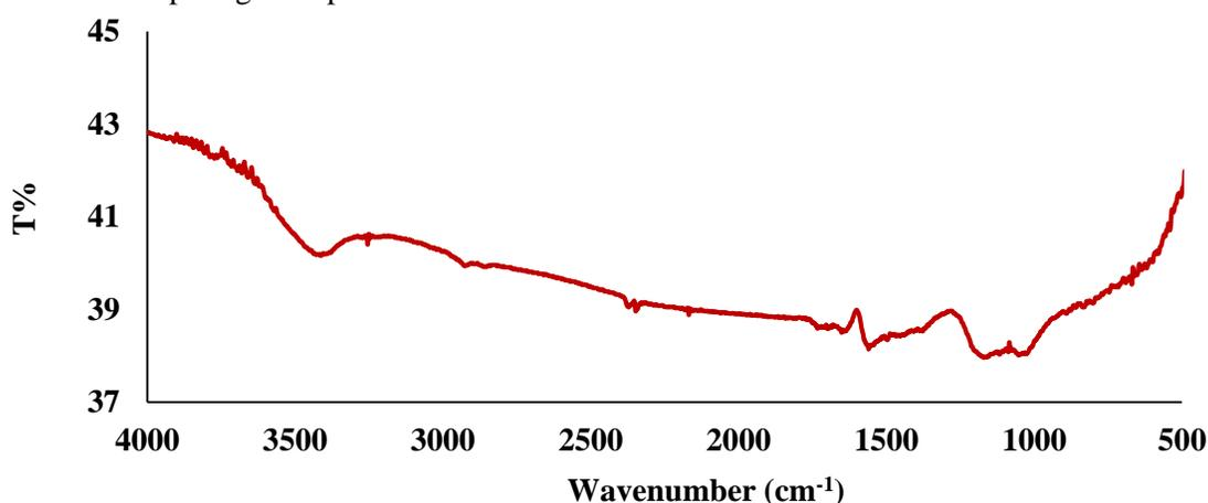
**Fig. 2.** FTIR spectrum of B-RGO
