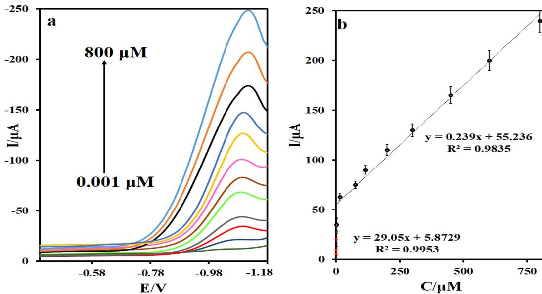
**Fig. 9.** (a) DPV of various concentrations of oxazepam on the B-RGO/Poly(ASP)|GCE surface under the optimal condition and (b) calibration curve
