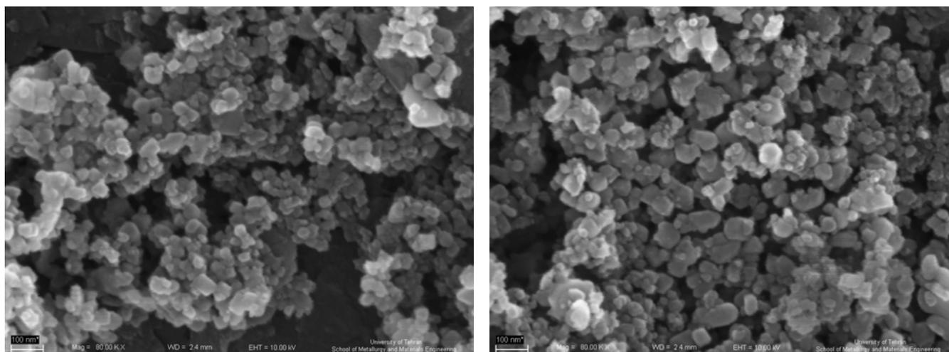
Fig. 2. FE-SEM micrographs of MgO nano-plates.
