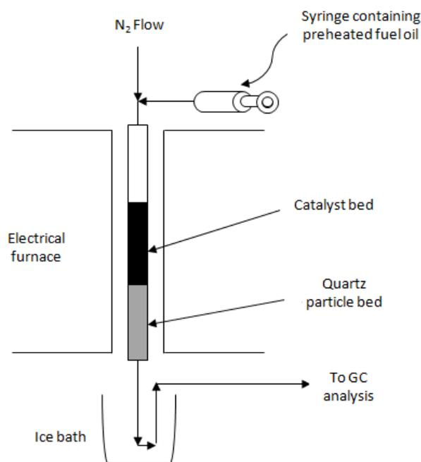
**Fig.4.** Schematic flow diagram of the experimental set-up.
