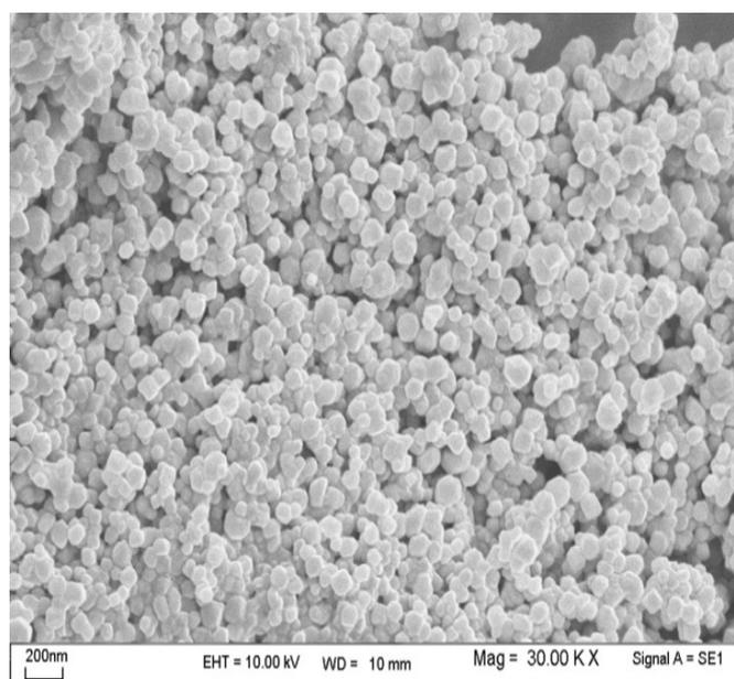
**Fig. 2.** SEM images of  $ZrP_2O_7$  NPs.
