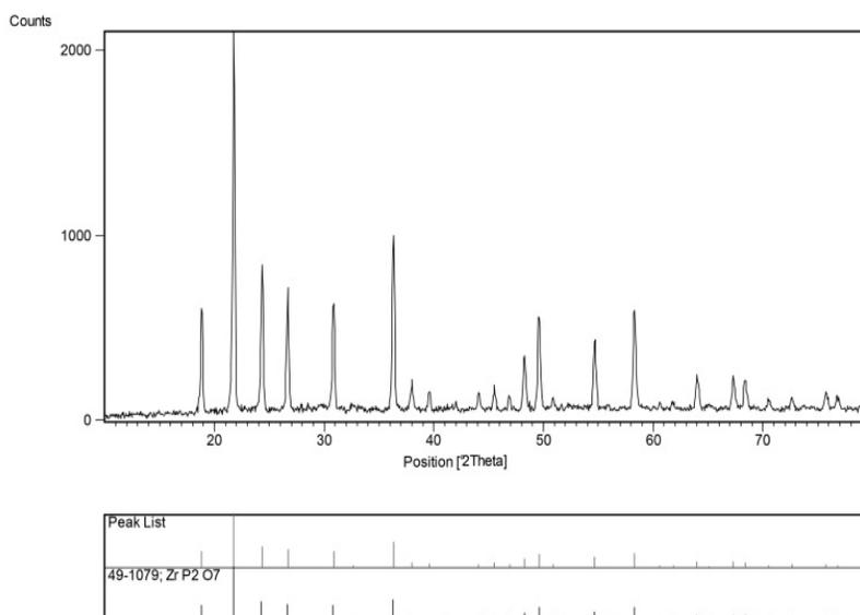
**Fig. 1.** The XRD pattern of  $ZrP_2O_7$  NPs.
