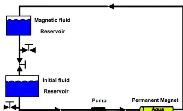
Fig. 1. The pilot of solvent magnetizing apparatus (SMA).
