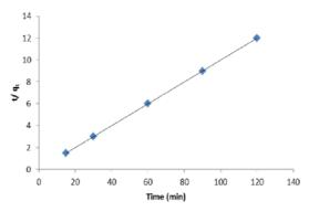
Figure 8: the pseudo second order model for dyed samples at the temperature, 100 °C
