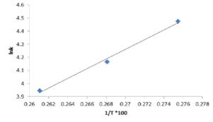
**Figure 10:** 1/T against lnk plotted to determine Thermodynamic parameters
