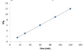
**Figure 7**: the pseudo second order model for dyed samples at the temperature, 90 C
