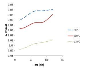
Figure 2: Effect of time on color adsorption at different temperatures.
