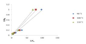
Figure 3: Langmuir adsorption isotherms at different temperatures.
