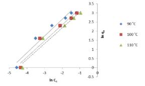
Figure 4: Freundlich adsorption isotherms at different temperatures.
