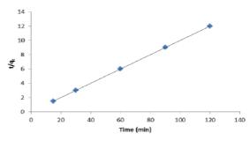
**Figure 9**: the pseudo second order model for dyed samples at the temperature,  $110^{\circ}$ C
