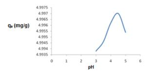
Figure 1: Effect of pH on dye adsorption.
