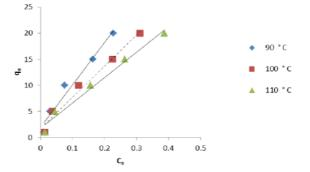
**Figure 5**: Nernst Adsorption isotherms for dyed samples at different temperatures.
