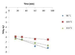
Figure 6: pseudo first equations for dyed samples at different temperatures
