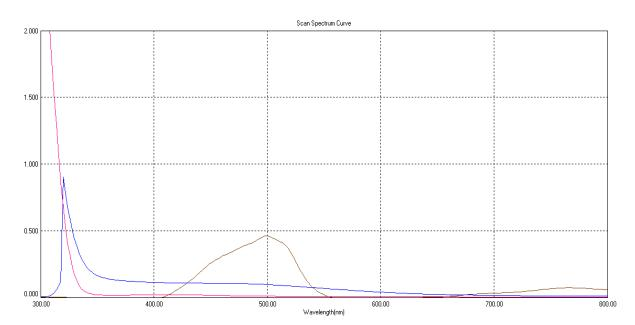
Figure 1: (A) The absorbance spectrum for the colored product figuration opposite the blank reagent solution (B) The absorbance spectrum for the solution of blank opposite deionized water(C) the absorbance spectrum of drug opposite ethanol solvent
