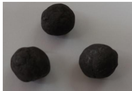
Figure 1: Image of iron ore pellet.
