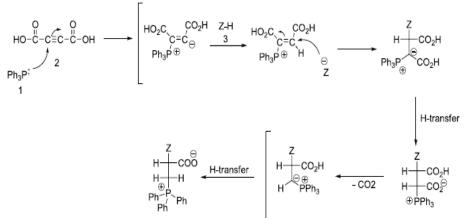
Figure 10: Proposed mechanism for the reaction between 1, 2 and 3 for generation of stable 1,5-diionic organophosphorus compound
