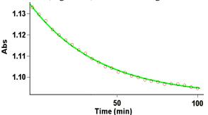
**Figure 9:** Pseudo first order fit curve (solid line) for the reaction in the presence of excess **1** ( $3 \times 10^{-2}$  M) at 378 nm and 25 °C in CH<sub>2</sub>Cl<sub>2</sub>.
