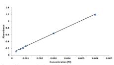
**Figure 6:** A linear relationship between concentrations and absorbance values at 378 nm for carbazole in  $CH_2Cl_2$  by the UV-vis spectrophotometer
