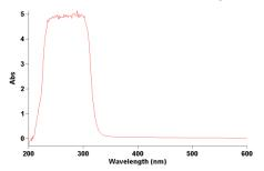
**Figure 2:** The UV spectrum of triphenylphosphine 1 ( $3 \times 10^{-3}$  M) in CH<sub>2</sub>Cl<sub>2</sub>
