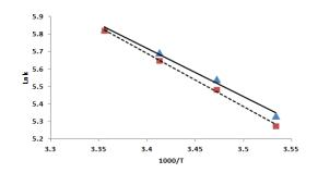
Figure 8: Dependence of second order rate constant (Ln  $k_2$ ) on reciprocal temperature for the reaction at 378 nm (solid line) and 358 nm (dash line) according with Arrhenius equation in CH<sub>2</sub>Cl<sub>2</sub>.
