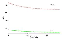
**Figure 7:** Experimental absorbance change (dotted line) accompanied with the second order fit curve (full line) against time at 358 and 378 nm for the reaction between 1, 2 and 3 in CH<sub>2</sub>Cl<sub>2</sub> at 25 °C
