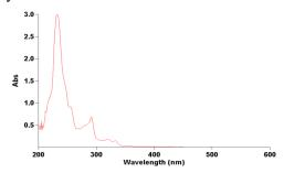
Figure 3: The UV spectrum of acetylenedicarboxylic acid (ADA)  $2 (3 \times 10^{-3} \text{M})$  in CH<sub>2</sub>Cl<sub>2</sub>
