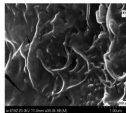
(A) Concrete with 0.5% weight fraction of MWCNTs
