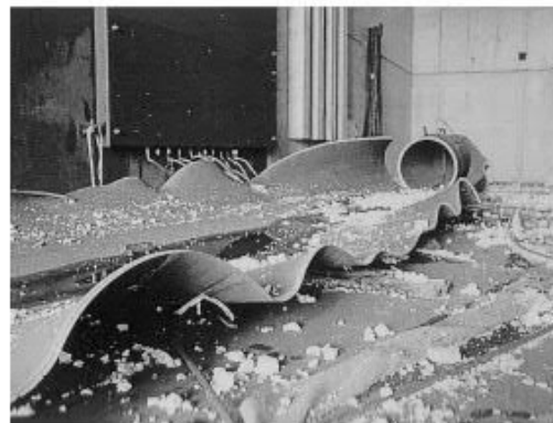
(b) after the burst test
