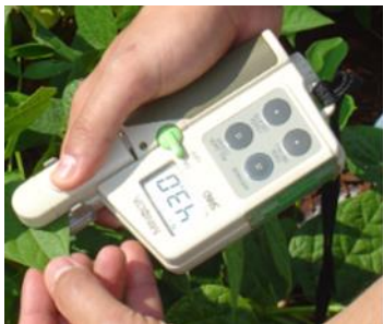
Fig 1- Laboratory steps: First, chlorophyll measurement in the middle and sample dryer in the oven at the end
