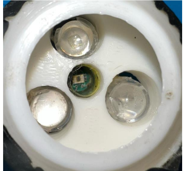
Fig. 4 Custom-Designed Mechanical Fixture for Sensor and LED Placement
