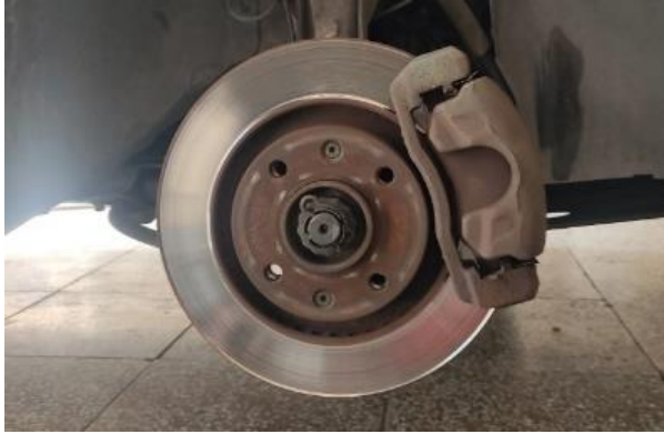
Fig. 3 Peugeot 206 brake disc and caliper.
