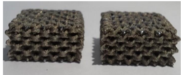
Fig. 12 Simple lattice structure after compressive test.
