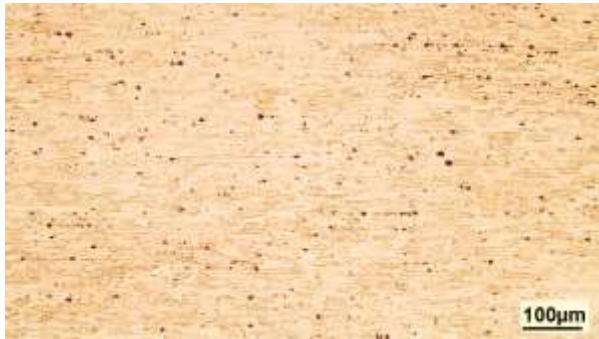
Fig. 8 Optical micrograph of the BM of AA specimen.
