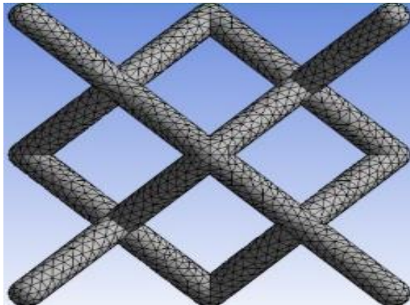
Fig. 6 4 Nodes rigid 3D shell mesh.
