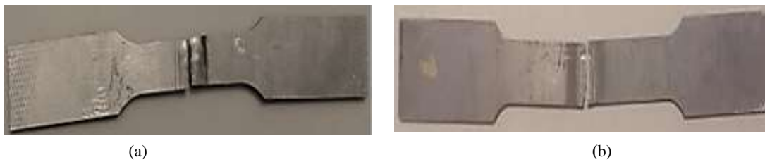
Fig. 12 Fractures in the weld zone of: (a): The WB, and (b): The AA specimens.
