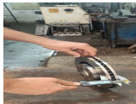
Fig. 2 Measurement of Peugeot 206 brake disc by caliper.
