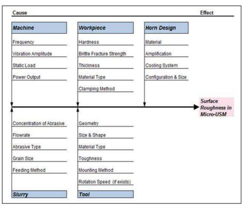
Figure1. Cause-and-effect diagram for surface roughness in micro-USM
