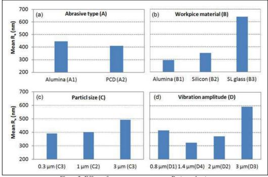
Figure 3. Effect of process parameters on R<sub>a</sub> (raw data)
