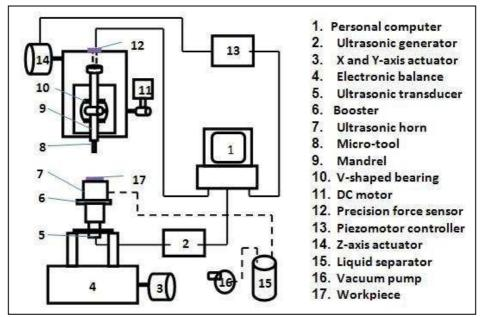
Figure2. Schematic diagram of in-house developed micro-USM system
