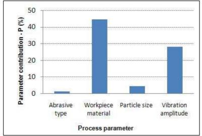
Figure 5. Percentage contribution of various parameters to surface roughness
