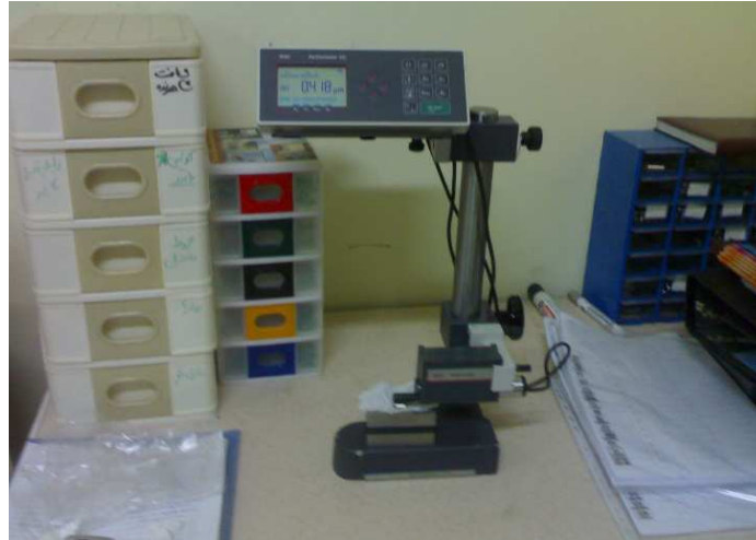
Fig.4. the method of measuring the surface roughness
