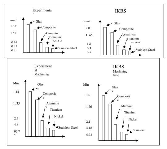
Figure 8. Comparison between IKBS cutting rate and experimental
