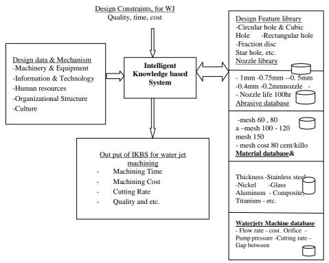
Figure6. Architecture of IKBS for water jet machining
