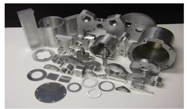
Figure 5. Examples parts machined by water jet
