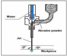
Figure1. A typical water jet head
