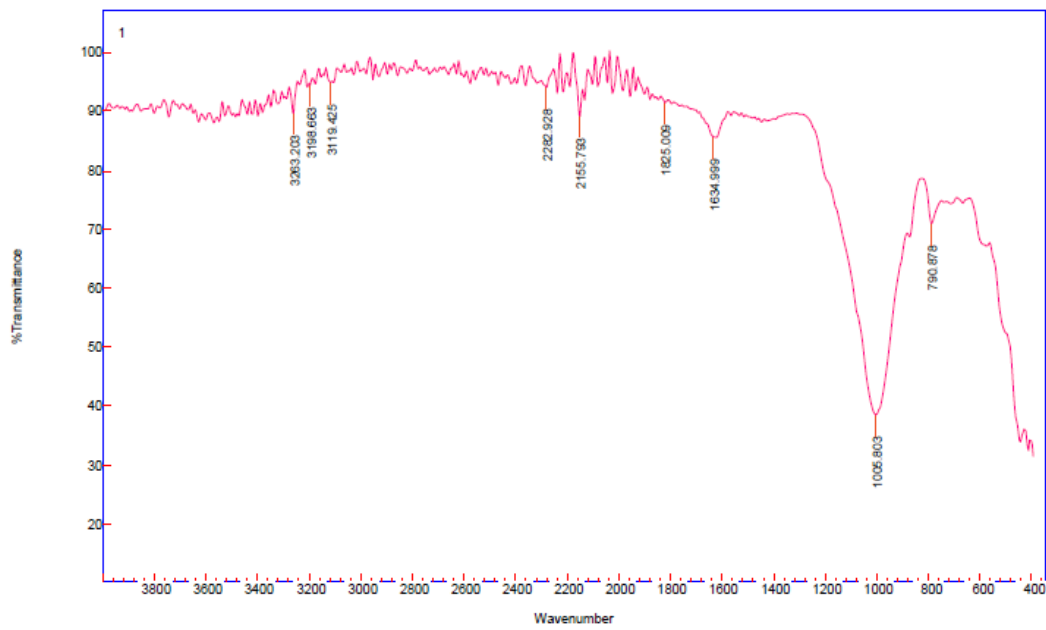
Figure 10. FTIR transmission spectrum of the natural zeolite (powder)
