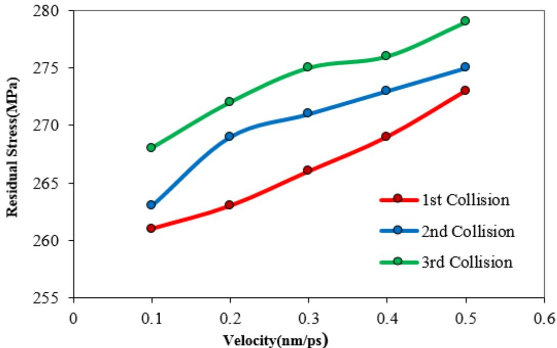
Figure. 4 The maximum residual stress of AZ31 atoms as a function of particle velocity
