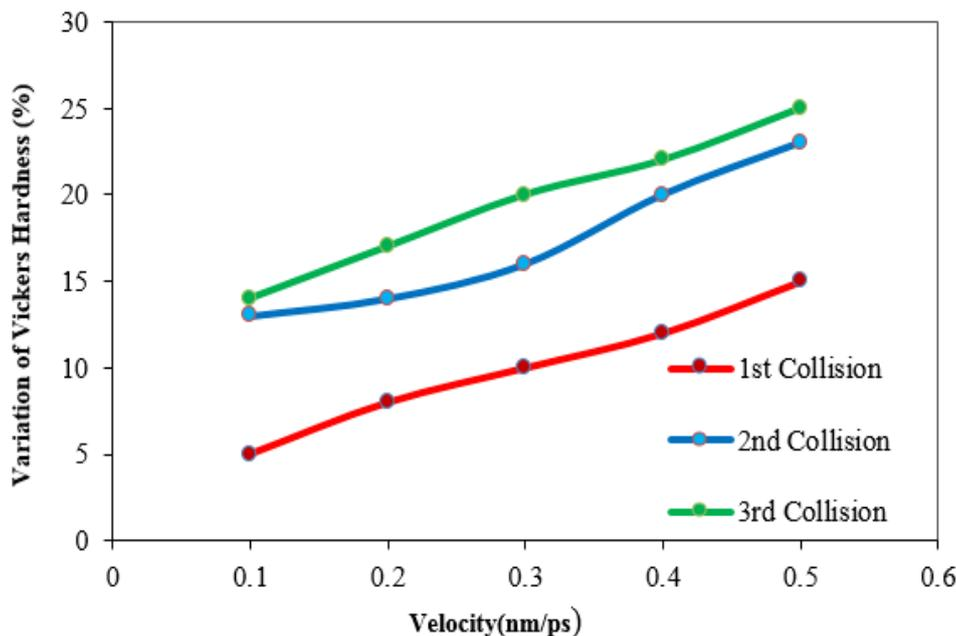
Figure 6. Variation of Vickers hardness parameter as a function of particle velocity
