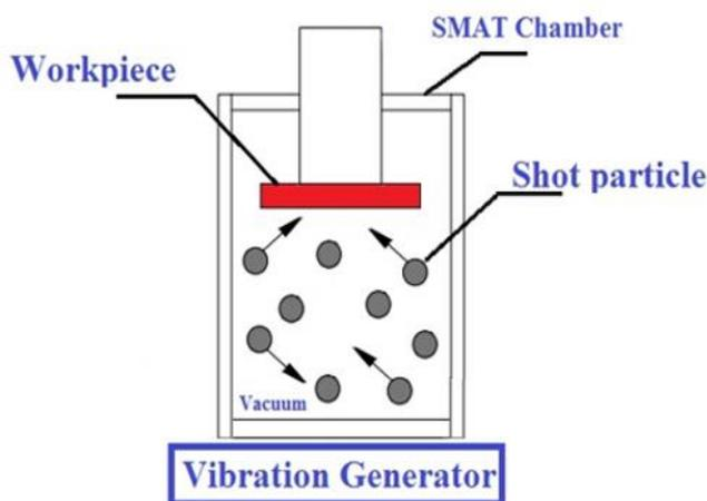
Figure 1. Schematic of the SMAT instrument
