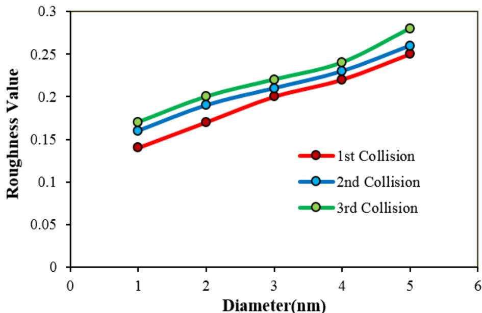
Figure 7. The roughness value of the AZ31 matrix as a function of particle size
