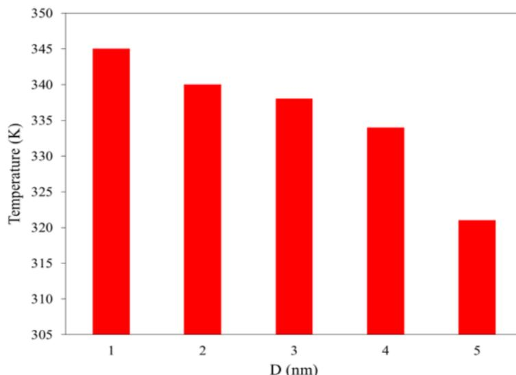
Figure 5. The maximum temperature of the AZ31 matrix after the third collision process as a function of colliding particle size
