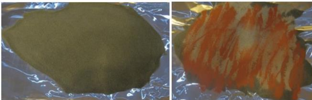
Figure 1. The photograph of produced Zink powder and added metal powders
