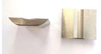
Figure5. Specimen prepared for the micro-hardness test
