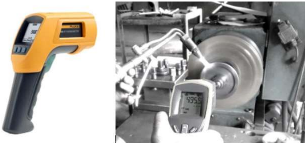
Figure6. FLUKE 568 thermo-Laser instrument and temperature control method
