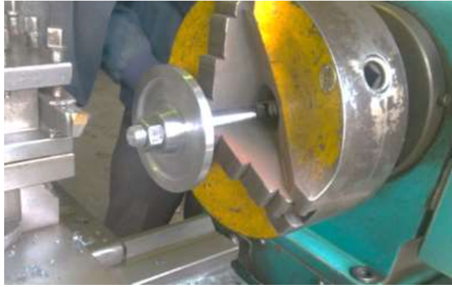
Figure4. The placement of disk on the shaft and their location on drilling chuck
