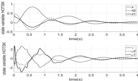
Fig. 4. State variables of the DPIC with a high-order fuzzy controller assuming  $\theta_1 = 20^\circ, \theta_2 = 20^\circ$
