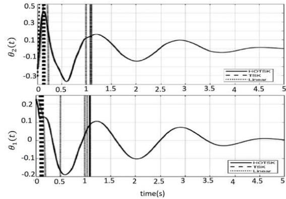
Fig. 6. A comparison of the deviation angles of the DPIC (with linear, zero- and first-order fuzzy, and high-order fuzzy controllers) with an initial deviation of  $\theta_1 = 15^\circ, \theta_2 = -15^\circ$
