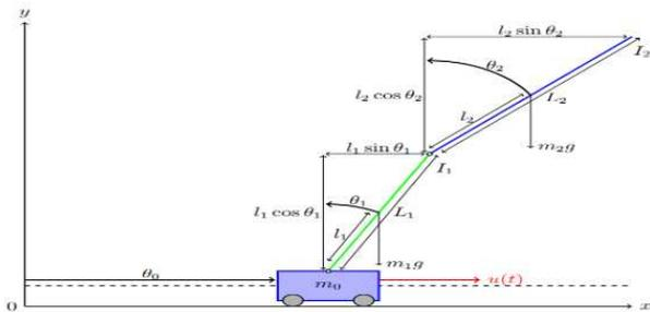
Fig. 2. Double pendulum inverted on a cart
