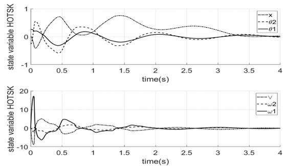
Fig. 7. State variables of the DPIC with a high-order fuzzy controller assuming  $\theta_1 = 15^\circ, \theta_2 = -15^\circ$
