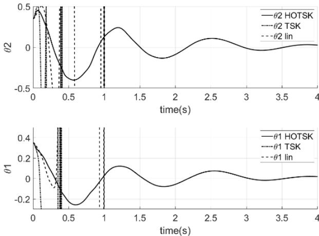
Fig. 3. A comparison of the deviation angles of the DPIC (with linear, zero- and first-order fuzzy, and high-order fuzzy controllers) with an initial deviation of  $\theta_1 = 20^\circ, \theta_2 = 20^\circ$
