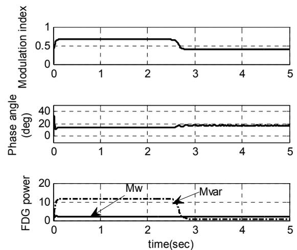
**Fig. 9:** Waveforms of modulation index, FDG voltage phase angel (on converter side), active and reactive power of FDG during start-up
