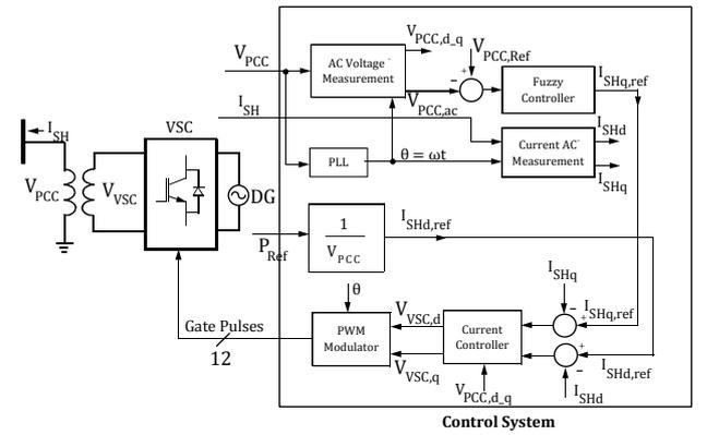
Fig. 4. The block diagram of voltage source converter control system
