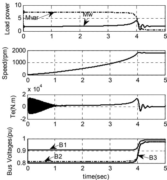
Fig. 7: Industrial load powers (MW & MVAR), motor speed (rpm), motor electromagnetic torque (Te), voltage profile of buses (pu) during start-up without FDG
