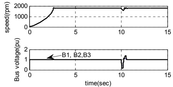
**Fig. 14:** Motor speed (rpm), voltage profile of buses (pu) during short-circuit with FDG
