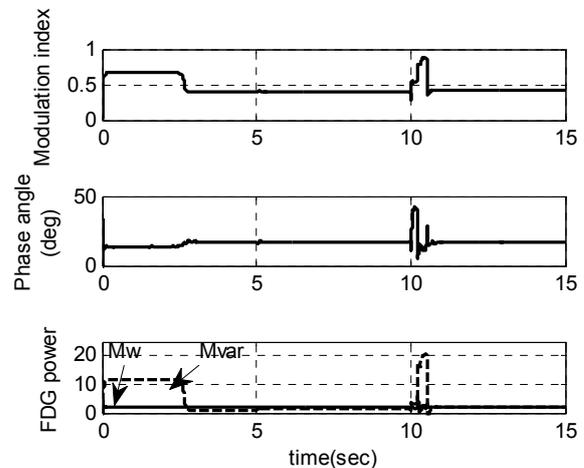
**Fig. 15:** Waveforms of modulation index, FDG voltage phase angel (on converter side), active and reactive power of FDG during short-circuit
