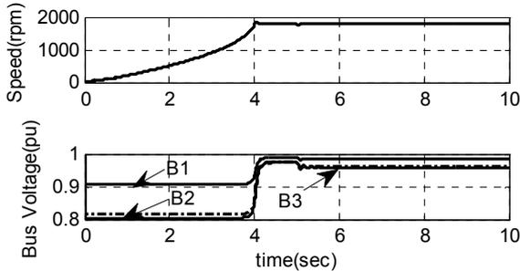
**Fig. 10:** Motor speed (rpm), voltage profile of buses (pu) during loading time without FDG
