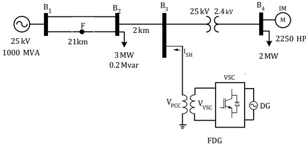
Fig. 1. Single line diagram of the system under test with FDG
