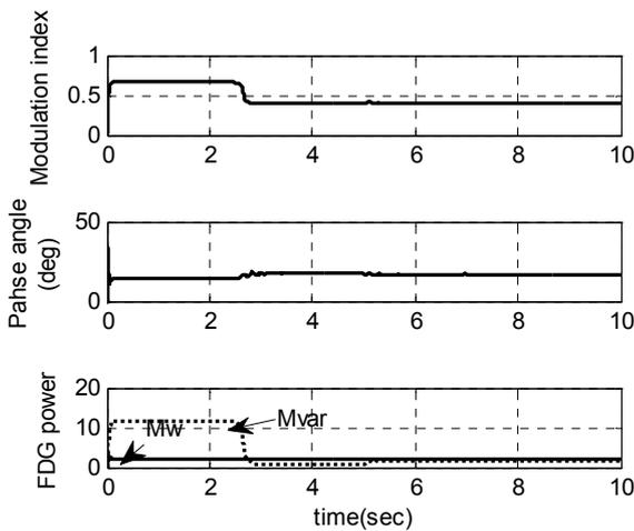
**Fig. 12:** Waveforms of modulation index, FDG voltage phase angel (on converter side), active and reactive power of FDG during loading time
