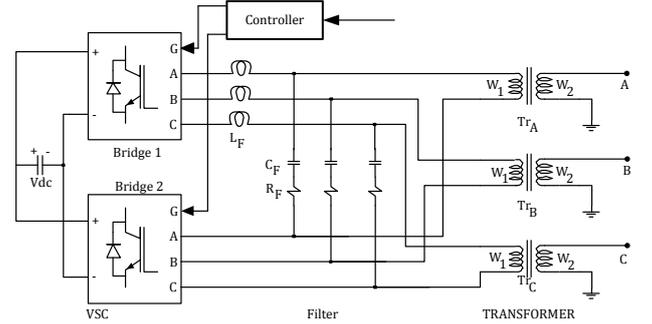
Fig. 2. Voltage source converter configuration
