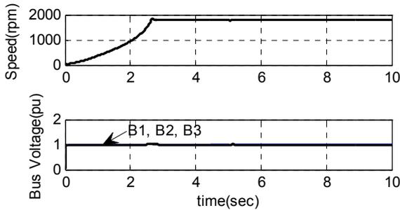
**Fig. 11:** Motor speed (rpm), voltage profile of buses (pu) during loading time with FDG
