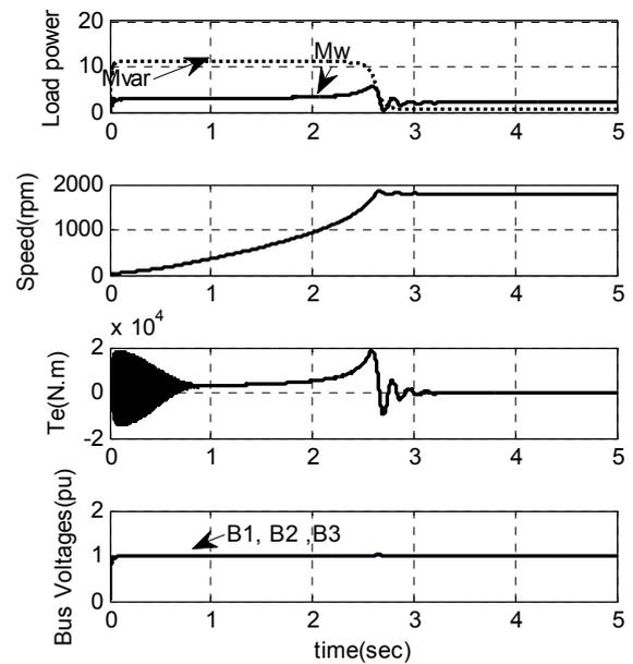
Fig. 8: Industrial load powers (MW & MVAR), motor speed (rpm), motor electromagnetic torque (Te), voltage profile of buses (pu) during start-up with FDG
