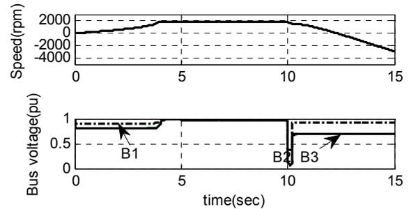
**Fig. 13:** Motor speed (rpm), voltage profile of buses (pu) during short-circuit without FDG
