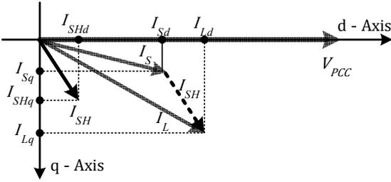
Fig. 3. Phasor diagram of FDG and load currents in dq reference frame
