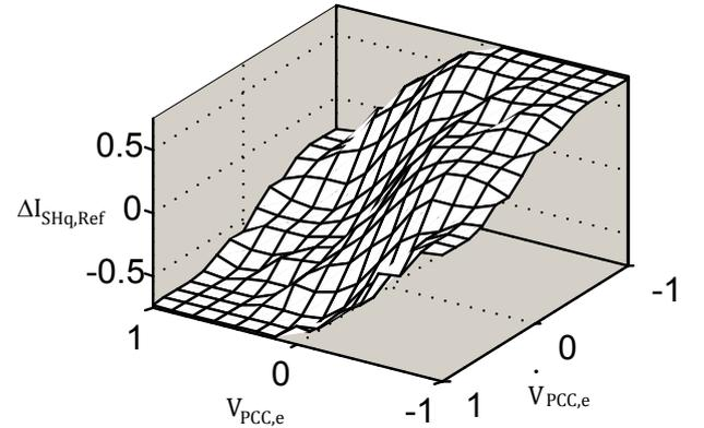
Fig. 6: Decision making space of common point voltage fuzzy controller
